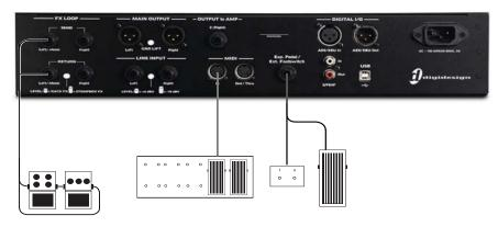
Figure 7. Effects and foot controller connections
