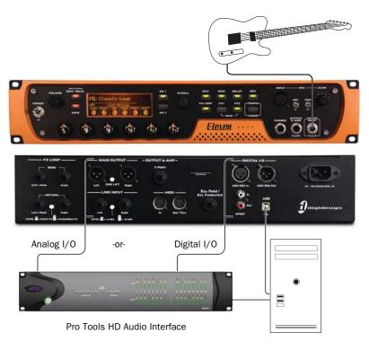
Figure 9. Eleven Rack connected to a Pro Tools | HD system
